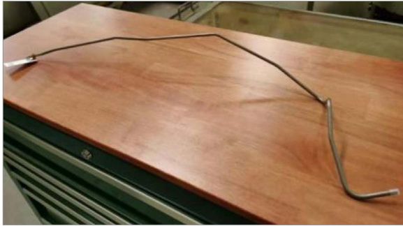
图 10 典型钛合金导管 Fig.10 Typical titanium alloy tube part
